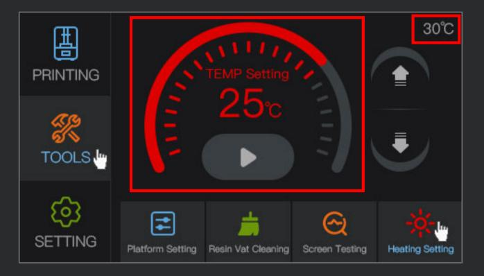
The printer's heating function is typically used in low-temperature environments. This function is not required at normal ambient temperatures. The heating temperature can be set between 20 and 40°C, with 30°C being the ideal option. Users can set the appropriate heating temperature based on the current ambient temperature.
