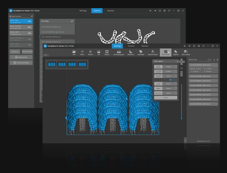
Auto hollowing and filling: Hollow out the inside of dental model and fill to reduce material consumption
